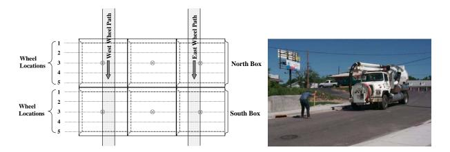
Figure 12. LVDT Layout and Axles Locations
