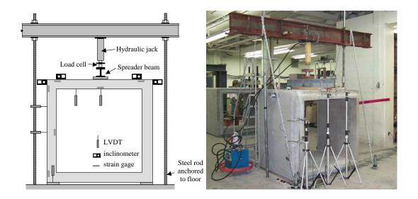
Figure 6. Test setup and instrumentation
