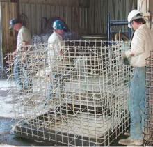
Figure 2. Rig for GFRP cage assembly
