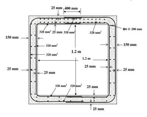
Figure 1. Details and reinforcement of GFRP reinforced box culvert.
