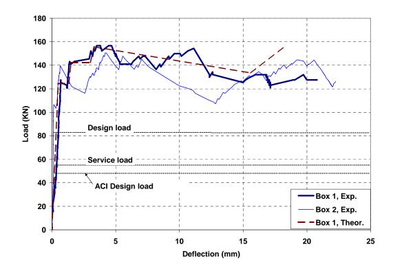
Figure 9. Comparison of experimental and theoretical load-deflection behavior
